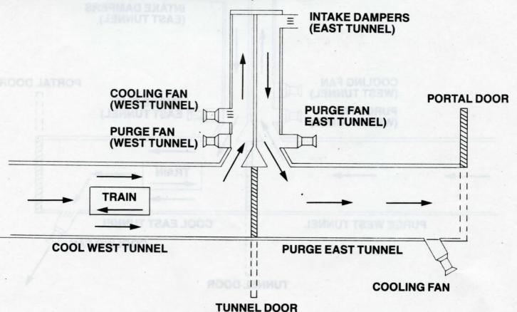
NOTE: PURGE OF EAST TUNNEL BEGINS WHEN REAR OF TRAIN PASSES SHAFT AND TUNNEL DOOR IS CLOSED BEHIND IT.
