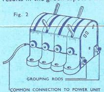
In most layouts the electrically-operated accessories will be controlled by individual Switches, which should be "banked" together as shown in Fig. 2. For this purpose Switch Grouping Rods, to take up to four or six Switches, are available. The G3 Switch referred to in this leaflet is similar in size and style to the D1 and D2 Switches used for other Hornby-Dublo purposes, and the three types of Switch can be grouped together. They are easily distinguishable as the D1 Switch has a red case,
