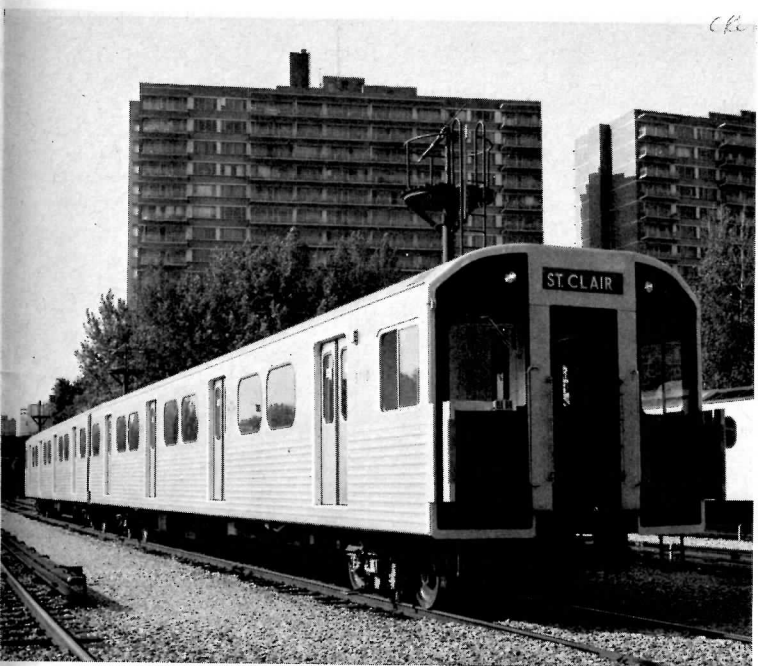
TOP LEFT: PCC 4520 underground at St. Clair West Station on the Spadina Subway. (T. Wickson). TOP RIGHT: Interior of Glencairn Station. October 4 1977. (T. Wickson). LEFT: 2 car train of H5 Class Subway cars at Davisville Yard. Not all the cars have yet been delivered and already, there has been a change: The black paint on the front of the cars is being dispensed with, as they are too hard to see in tunnels. (TTC). BELOW LEFT: 5 October 1977 saw a special train consisting of 2 H class cars and locomotive RT18 to take the TTC Commissioners on a tour of the Spadina line. Northbound approaching Lawrence West Station. BELOW RIGHT: The special train at Lawrence West Station. Both photos T. Wickson.
