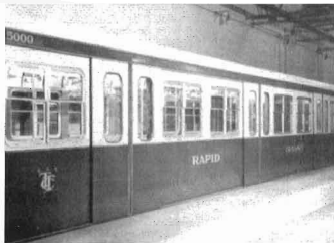
This "mock up" of a subway car was built late in 1949 to test the door and window arrangements before the actual cars were ordered. No passenger would be more than 7 feet 6 inches from a door.
