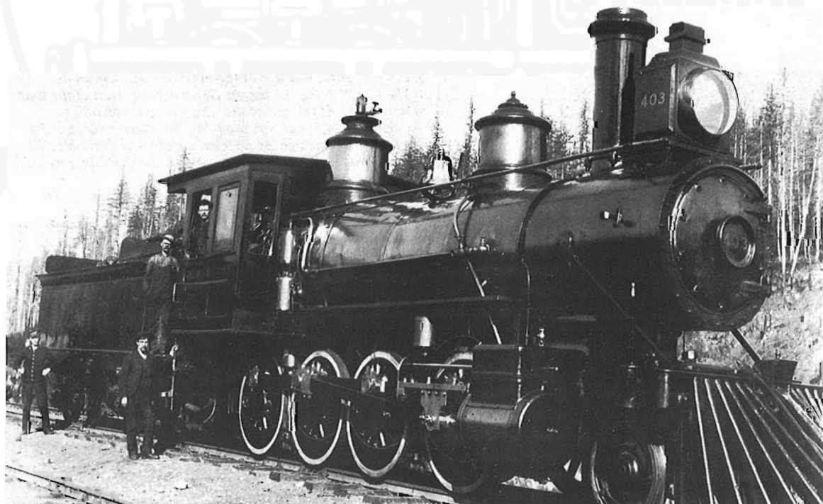
Canadian Pacific Ry class SD 2-8-0 steam locomotive no. 403, built in 1886 and assigned to the Pacific Division. Photo taken circa 1888.
