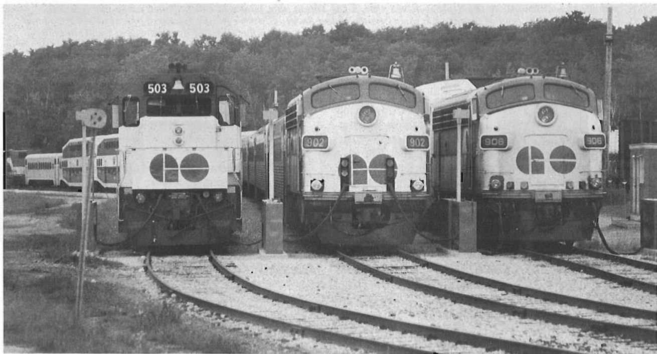
The three daily Toronto-Milton GO trains layover at Guelph Junction. In this August 1986 view are two generations of diesel power. GP40TC #503 is one of the 8 original locomotives bought for the start-up of GO in 1966. APU's 902 and 906, converted from FP7A's, were originally purchased by the Ontario Northland in 1952. On GO Transit, these units serve as auxillary power cars to generate the electricity to operate the services on the coaches, and as control cabs for push-pull operation.
