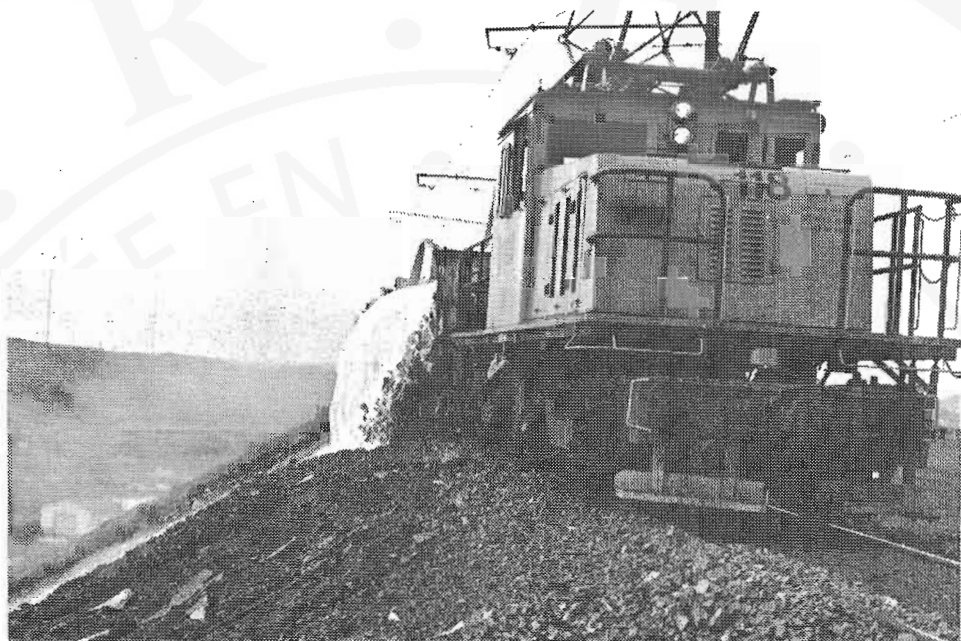
INCO Railway No. 118 at the head of a train from which molten slag is being poured at a temperature of 1600 degrees Farenheit. One can feel the heat from 100 feet away.
