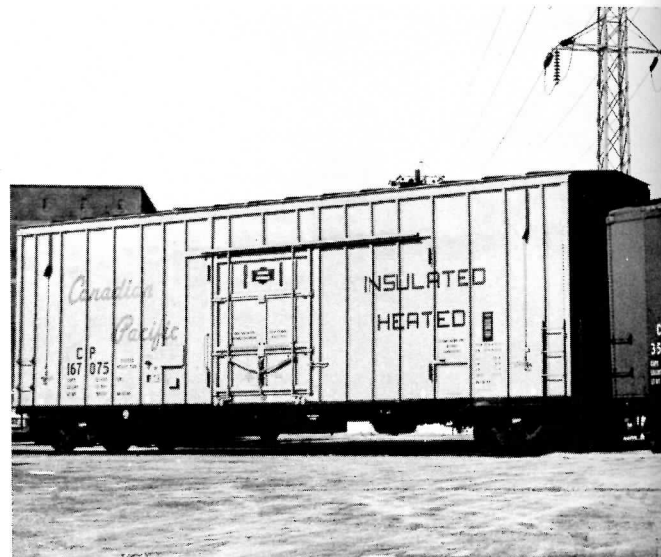
CP Rail has doubled the capacity of 25 insulated heated boxcars by raising their roofs two feet six inches. The modified cars are used to transport beer from Montreal to Quebec City, Hull and Sherbrooke. -- CP Rail.
