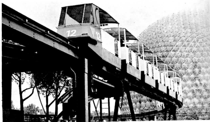
ABOVE: A minirail train passes a switch, whose position can be changed by rotating the curved segment (below the car) into operating position.
