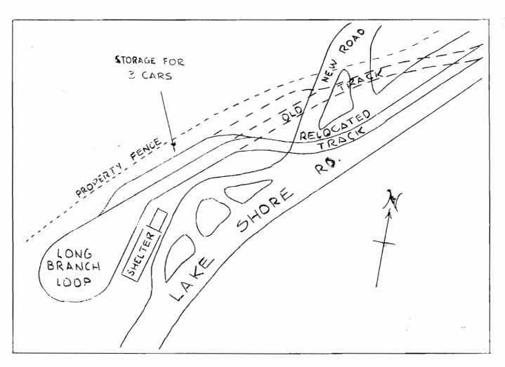
Track on the new alignment was connected up for use on the night of November 8-9. Track on the old alignment was subsequently lifted.
