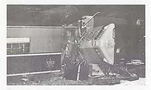
LEFT: GTW 4932, shown here, was the leading unit when train No. 6 derailed at Rexdale, Ont. Its train actually collided with it, the motion of the cars causing the damage.
