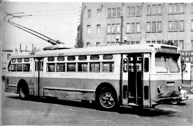
Valparaiso (Chile) trolley bus #717. This was a Pullman Standard Model 700 (48 seats) built in 1954. This was Pullman's last model before the discontinuance of Trolley Bus production. It was never sold in North America and was probably built in Chile under licence.
