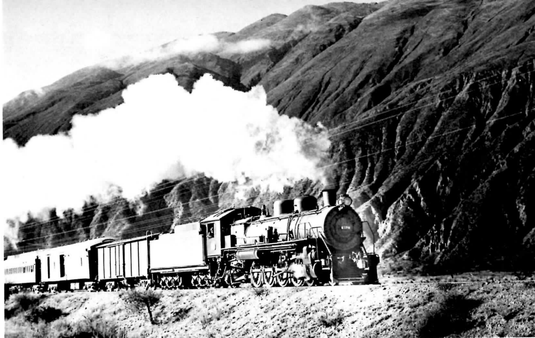
Southbound with a passenger train heading for Jujuy on F.C. General Belgrano. The locomotive is a light meter gauge 4-8-2 #862. July 1972
