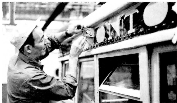
UPPER: Each letter making up, "TORONTO TRANSPORTATION COMMISSION", is carefully traced and cut from a clear masking tape spread along the letterboard.
