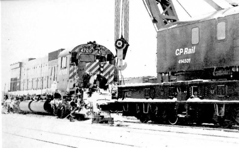
Oops! CP Rail M636 #4700 stubbed her toe on an ice-packed switch at the west end of West Toronto Yard, March 18, 1973. Crane 414501 was called to the scene to remedy the situation. (Robbin Rekiel)
