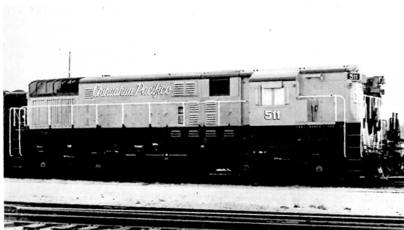
Chihuahua Pacific H16-44 seen at Toronto Yard, April 9th, 1973, after rebuilding and repainting at United Railway Supply in Montreal. Other CHP units rebuilt at URS include 501-525 and 600-604. (Robbin Rekiel)
