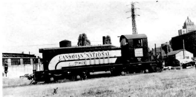
TOP RIGHT:MLW S2 7976 was built June 1949,in black and orange-yellow, sans Canadian National herald on the cab,in keeping with the rest of the MLW built switchers.Renumbered 8123,the loco was retired Apr.71. ABOVE RIGHT:EMD NW2 7963 was built December 1947,Class Q-5-A.Reclassified as GS10a,the engine was sold May 1969 to PNC and was rebuilt and resold to US Steel Gary Works #33.(JTA SMITH/UCRS)
