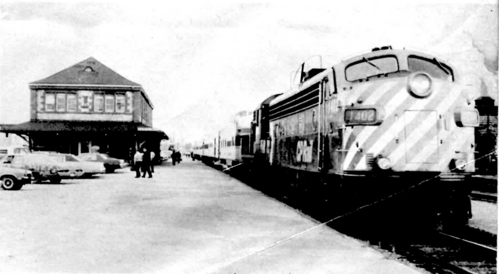
The Montreal section of the Canadian pauses briefly on its run to the west at North Bay to pick up passengers and change crews. During the stop the locomotives will also be refuelled and the water tanks for the steam generators topped up. (R.G. Eastman)
