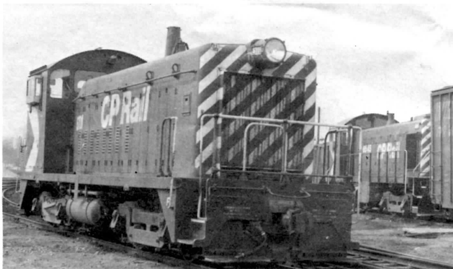
ABOVE: Canadian Pacific 6701 (DS8a, GMD SW8 b1t 1950 along with 6545 (DS6e, MLW S5, 1955) both working the London Quebec Street Facility. 10 April 1978 (I.C. Platt) BELOW: CP 7025 (DS10c, ALCO S2 B1t 1945) working the Smiths' Falls Yard 28 June 78 (I.C. Platt)
