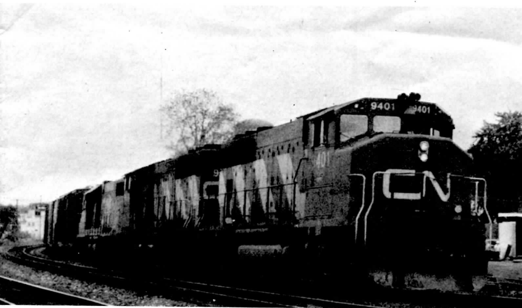
A pair of wide nose GP40-2(W)'s 9401 and 9416 leading GP38-2 5511 on a westbound hotshot near Napanee Ontario 28 June 78. (I.C.Platt)
