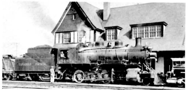
Canadian Pacific 2-8-0 3487, working a ballast train, was built by Montreal Locomotive Works as a part of class m-4-g in 1907. (JTA SMITH/UCRS)
