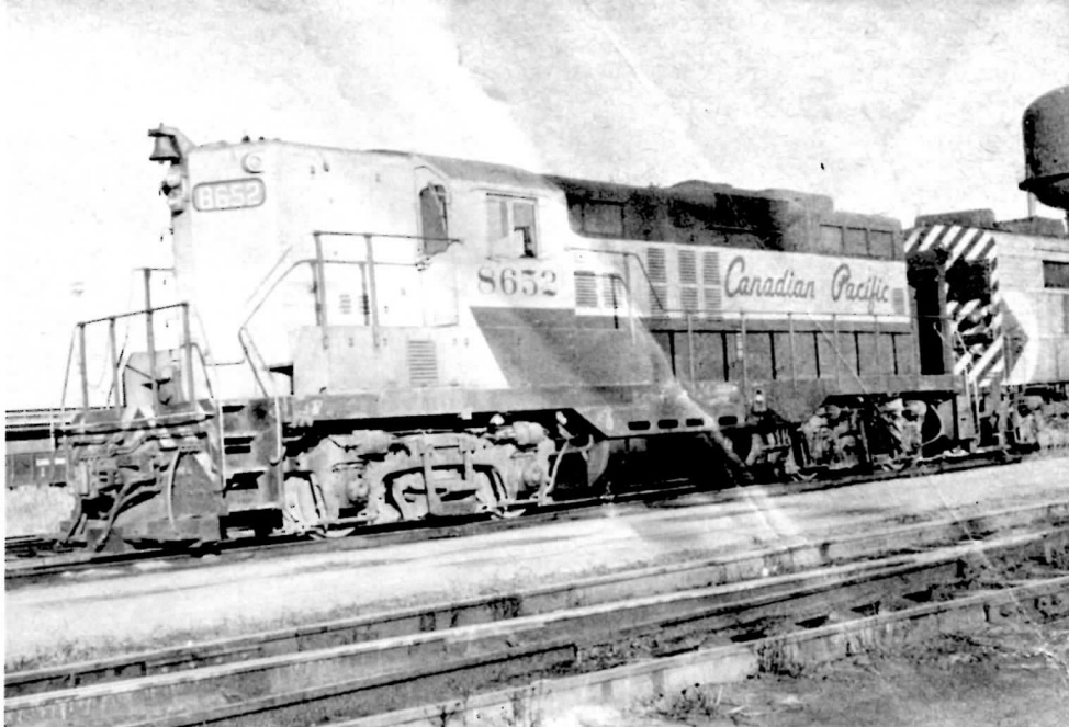
Canadian Pacific GP9 8652, road class DRS 17d was built by GMD 1957 rated 1750 hp, except in freight service when they are rated at 1600. Taken 26 November 1973 at St. Luc Pierre Patenaude.
