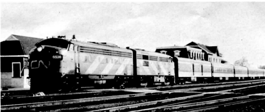
LEFT: Two locomotives, two builders-GMD built FP9A 6535 and FPA4 6786 eastbound in front of the Belleville Station May 1974. Ironically, this was the last train over the CN from Toronto prior to the wreck referred to in the top photo. (RWL) BELOW: VIA units 6524-6540 at Montreal Yard on 30-10-77. Note variations on both units as to roof details, with the blue extending into the filter grills on 6540, black on top of nose is different as well as the location of the VIA logo on both units. (Pierre Patenaude)
