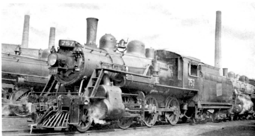
ABOVE: Built for the Montreal-lakeshore Commuter service by the Montreal Locomotive Works for the Grand Trunk, 4-6-4T #50 became CN Class X-10-a. It was retired and scrapped in 1960. (JTA SMITH/UCRS) RIGHT: 2-6-0 757 on the ready track. The engine was built by the GTR 1902 as 1220. Classed as E-7-a by the CN, it was withdrawn and scrapped December 1947. (JTA SMITH/UCRS) BELOW: Freshly shopped and painted, 2-8-0 2378 was built by Canadian Locomotive Company at Kingston for the Canadian Government Railways as #310. (JTA SMITH/UCRS)
