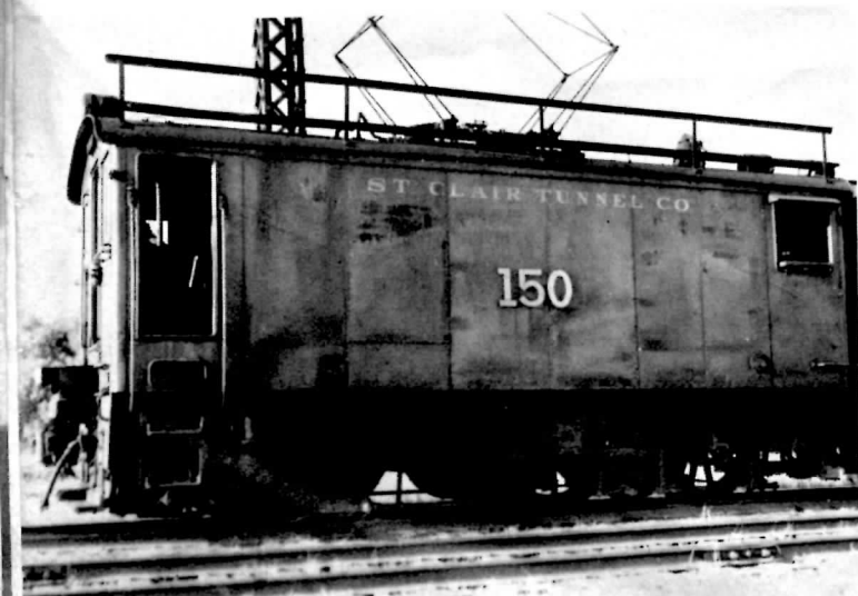
LEFT AND RIGHT:St.Clair Tunnel Company box cab electrics were used in the steam era to haul trains between Sarnia Ontario and Port Huron Michigan,and replaced a series of 0-8-0 Tank engines.Both 150 and 153 were built by Baldwin/Westinghouse July 1908 as part of an order St Clair Tunnel Company 1310-05 in reverse order and were renumbered as Grand Trunk 2660-55,again in reverse order.Taken over by CN as 1950-55 in 1923, they were renumbered 150-55 and retired in 1959.(JTA$UCRS)
