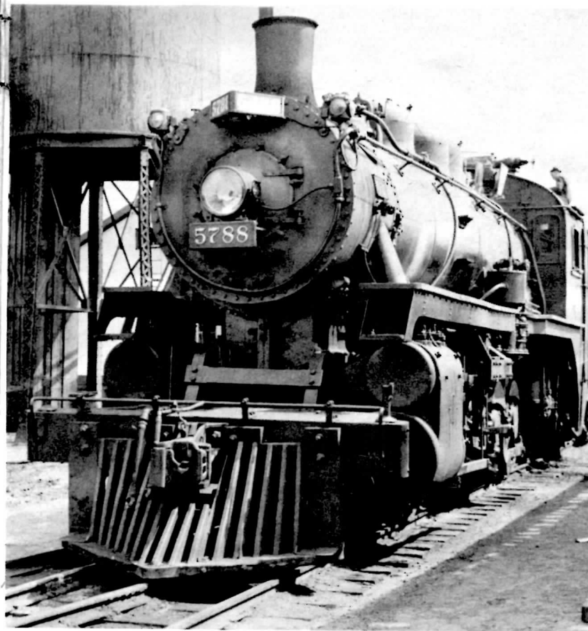
Canadian Pacific 2-10-0 5788 on the servicing tracks between runs at Kamloops British Columbia. The Class R-3-d was built by CPR in 1918. Taken Sept. 1943 (JTA SMITH/UCRS)
