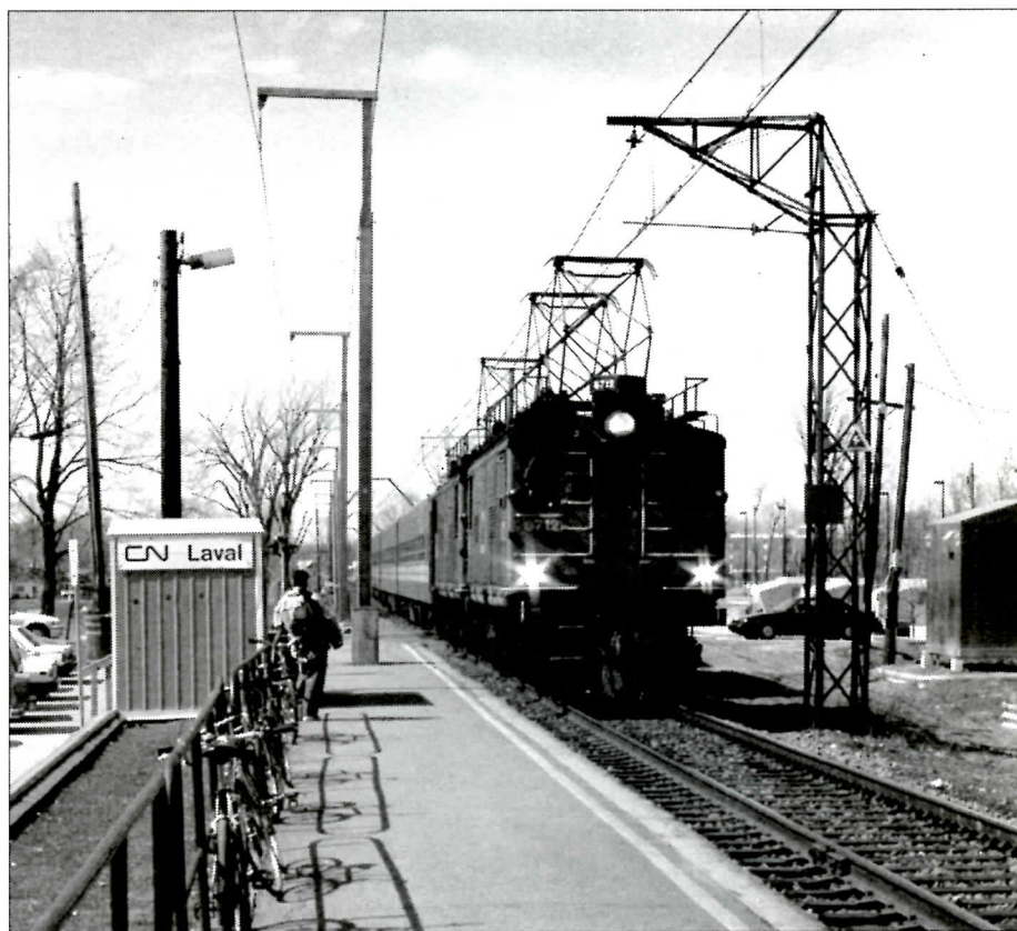
Above is a photo by Michel Belhumeur at Laval-sur-le-Lac station, showing a train typical of the Deux-Montagnes line towards the end of 2400 V DC operation. The 1914-era boxcab motors are hauling a train of comparatively-new 1950s coaches, leased from VIA and fitted with opening windows, to eliminate the need to maintain the on-board airconditioning. Also common during the rebuilding period was the sight of old and new plant; on the left are new masts, ready for the 25 kV AC catenary; on the right are the old lattice masts, from the original electrification of the line. This station was not rebuilt, and the new trains now pass this site without stopping.
