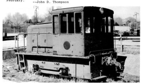
This General Electric 25-ton switcher was a familiar sight at the Davenport Works, Toronto, of Canadian General Electric. Built at GE's Erie plant in 1947, serial number 29226, it served the Toronto facility for some 40 years before retirement. Note the extended "link and pin" style coupler for moving special cars. The paint scheme was green body, orange truck.
