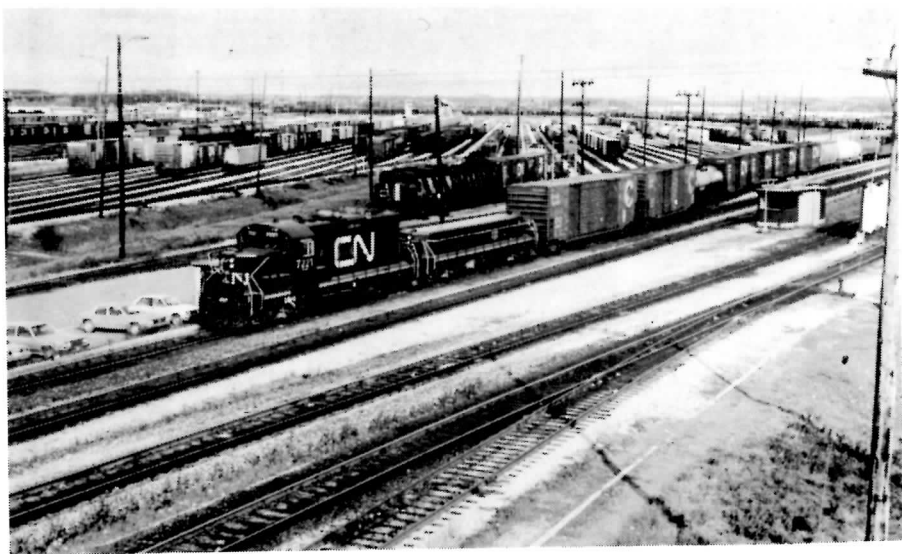
Among the more interesting motive power sights around Metro Toronto are CN's chop nosed Geeps and hump booster units, also known as 'slugs' or 'calves'. This combination of 7221 and 222 was photographed southbound on November 1, 1987.
