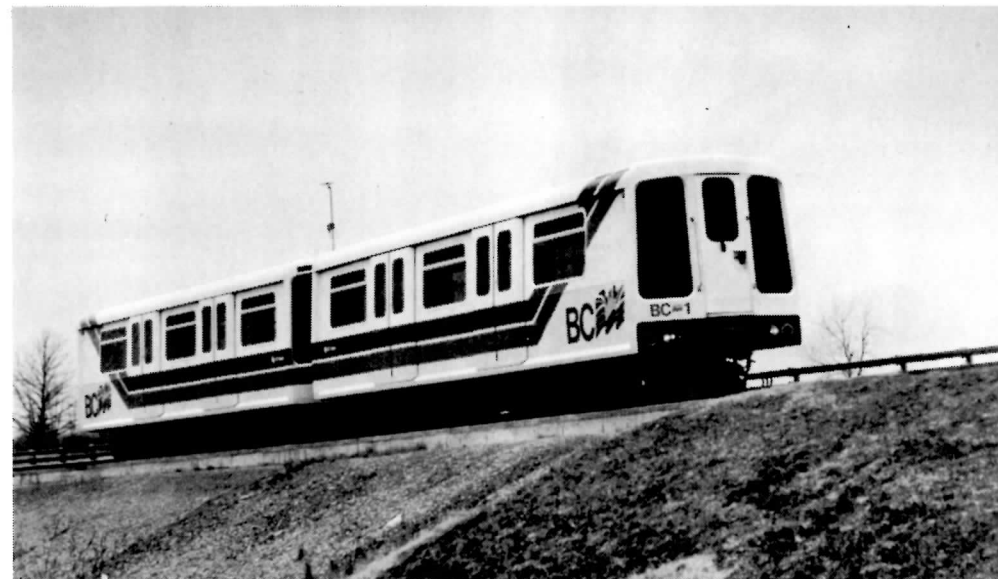
The first pair of completed ALRT cars for Vancouver are put through their paces at UTDC's Kingston test centre before being trucked out west in March, 1983. The 40-foot cars, similar to those ordered by the TTC for the Scarborough line, are white with red and blue stripes. The makeshift aerial on the first car is for radio contact. --TTC photo by Ted Wickson
