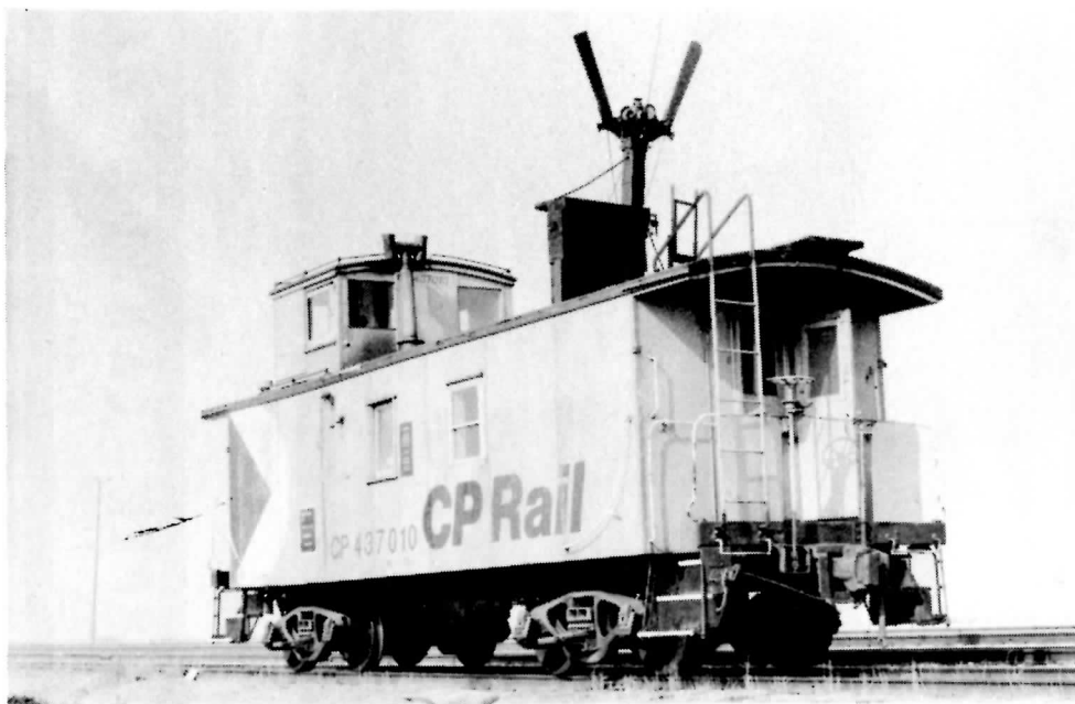
Would you believe it? CPR caboose 437010, based at Winnipeg, is used as a mobile train order office. A recent outing was during the installation of CWR on the Carberry Sub., when the unique vehicle protected the work train in the vicinity of Rosser, Man.
