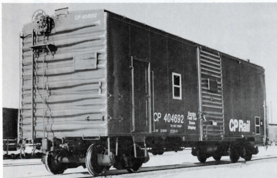
CP Rail 404692, a standard 40-foot box car which has been converted into a "Dome Instruction Car" for teaching employees tank car safety. The interior has been equipped with domes, valves, other fittings and cutaway displays to demonstrate the components of most tank cars used on this continent. One wall display relates to tank car placarding.
