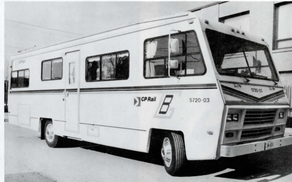
It may look like a rather undistinguished mobile home, but CP Rail unit 5720-03 will come to make an important contribution to the efficient handling of main line freight trains in Western Canada. Known as a train/dynamic analyser, the half-million dollar vehicle is used to instruct locomotive engineers in the operation of long and heavy trains.
